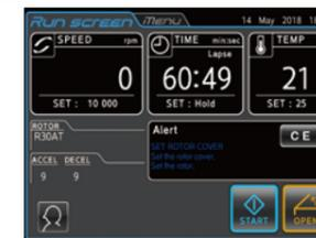
Rotor cover detection sensor prevents rotors from spinning without rotor covers.
